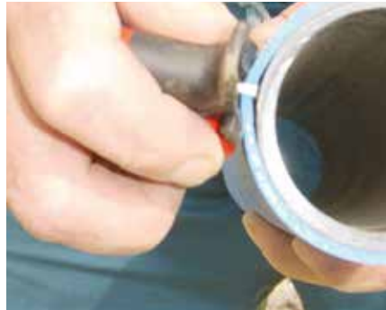
Place the cutting tool between the outer and inner layer.
